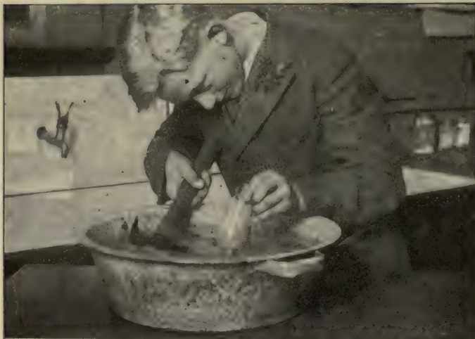
FIG. 4. When the point is knocked off the electric lamp, the water is forced into the vacuum.
